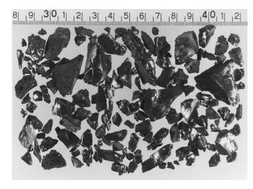
SEM Photomicrograph<sup>4)</sup> scale see photograph, Crystalline Boron Grade P1
