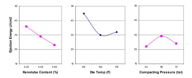
Figure 2: Effect of lubricant content, die temperature, and compacting pressure on the ejection energy of D.AE + 0.3%C
