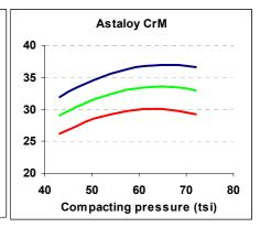
Figure 4: Ejection energies achieved using a die temperature of  $60^{\circ}\text{C}(140^{\circ}\text{F})$  and  $0.30 - 0.60^{\text{w}}/_{\text{o}}$  Kenolube
