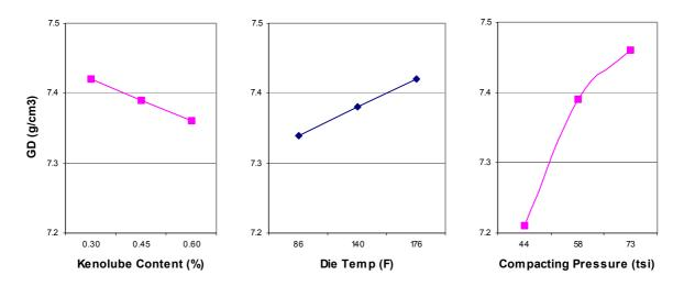
Figure 1: Effect of lubricant content, die temperature, and compacting pressure on the green density of D.AE + 0.3%C
