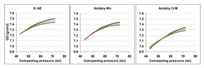
Figure 3: Green densities achievable using a die temperature of  $60^{\circ}$ C ( $140^{\circ}$ F) and  $0.30 - 0.60^{\text{w}}/_{\text{o}}$  Kenolube
