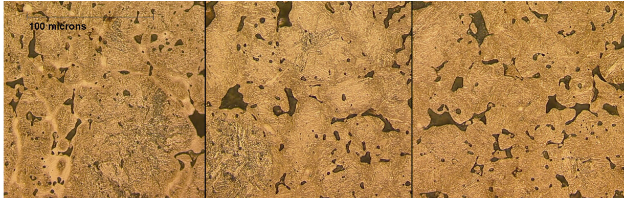
Figure 11a: CrL, sintered 10 min, 2.5°C/s cooling. Copper is concentrated in the grain boundaries.
