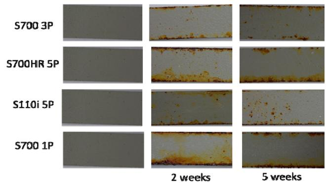
Fig. 8. Corroded samples with water-borne paint.
