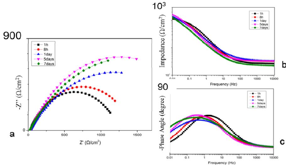
Figure 9. EIS spectra for untreated Somaloy 700 3P after exposure to 0.1 M NaCl solution: (a) Nyquist plot, (b) Impedance spectra and (c) Phase angle spectra.
