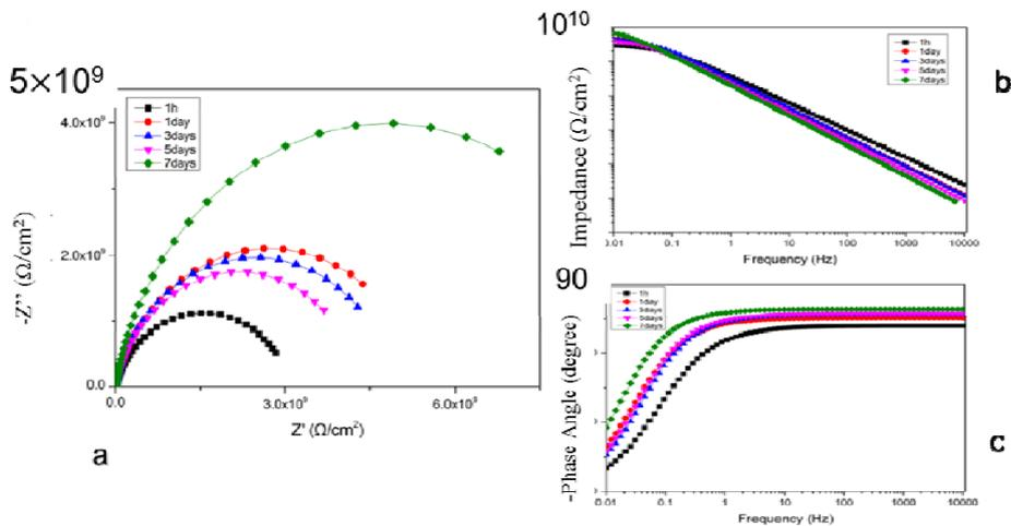
Figure 10 EIS spectra for Somaloy 700 3P with water-borne single coat paint after exposure to 0.1 M NaCl solution: (a) Nyquist plot, (b) Impedance spectra and (c) Phase angle spectra.
