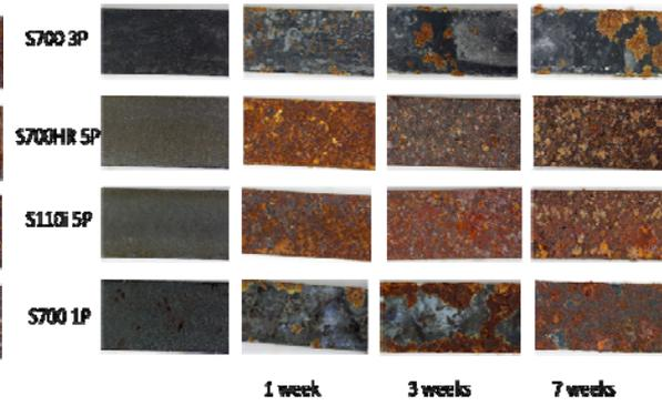
Fig. 6. Corroded samples with sodium silicate coating.
