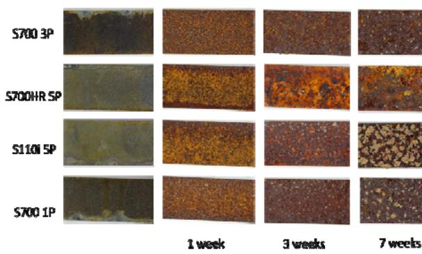
Fig. 5. Corroded samples with phosphate coating.
