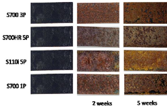
Fig. 7. Corroded samples with SCC3 coating.
