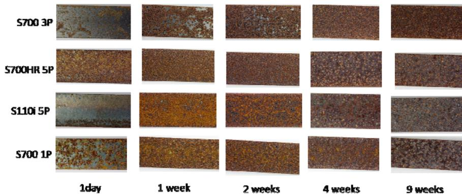
Figure 2. Photos of untreated Somaloy components corroded bar samples.
